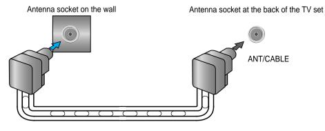
Feeder cable connection with the combined adapter
